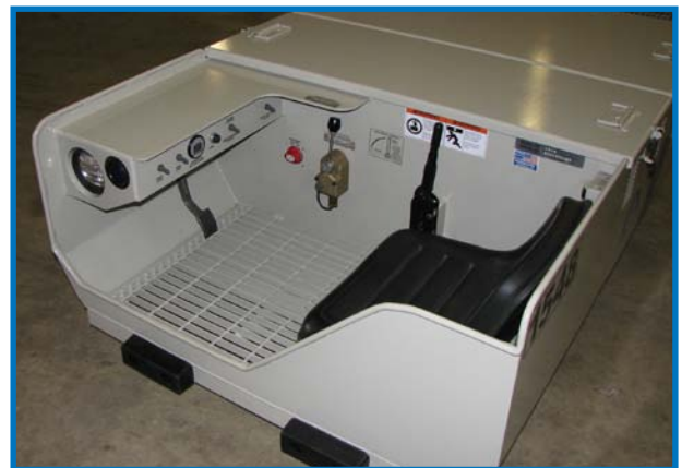
Operator Platform With Controls
