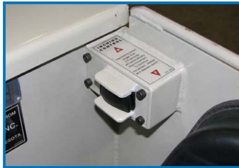
Removable main power switch to prevent accidental powering on of haul unit.
