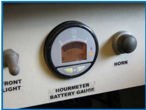
The battery gauge displays the battery charge level.
