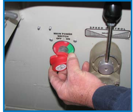
Removable main power switch to prevent accidental powering on of haul unit.
