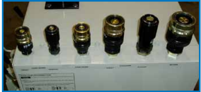
The quick couplers connect to the pressure, return, load sense, and case drain hydraulic hoses from the GBM P100Q Power Pack.
