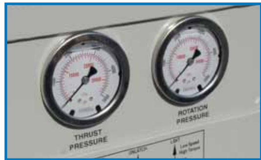
Hydraulic pressure gauges for monitoring thrust and rotation system pressures.
