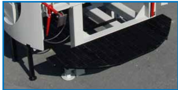
Operator platform located 18" above shaft floor provides firm footing to keep the operators above the water and mud.
