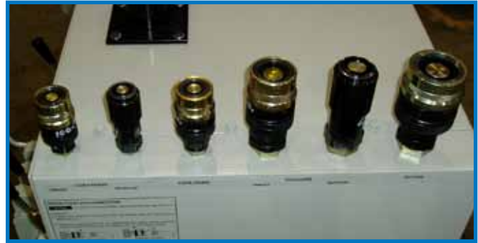
The quick couplers connect to the pressure, return, load sense and case drain hydraulic hoses from the GBM P100Q or P150Q Power Pack.
