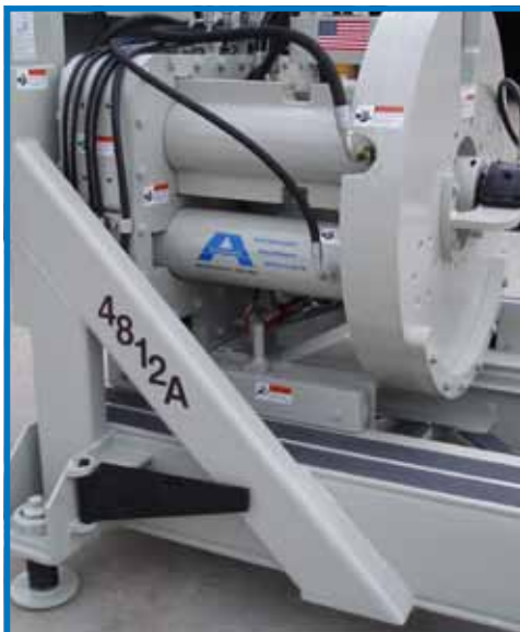
Four cylinders provide up to 200 ton thrust capacity.
