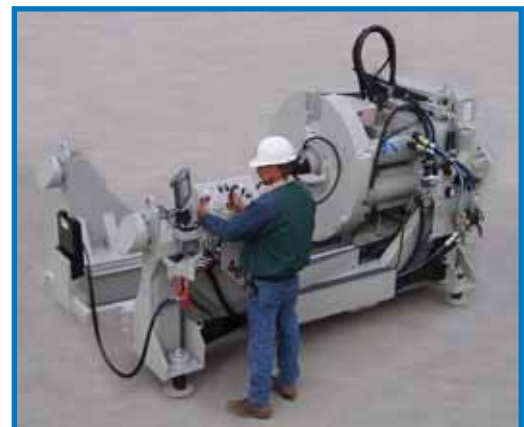
Operator control center for ease of operating and monitoring of system pressures.
