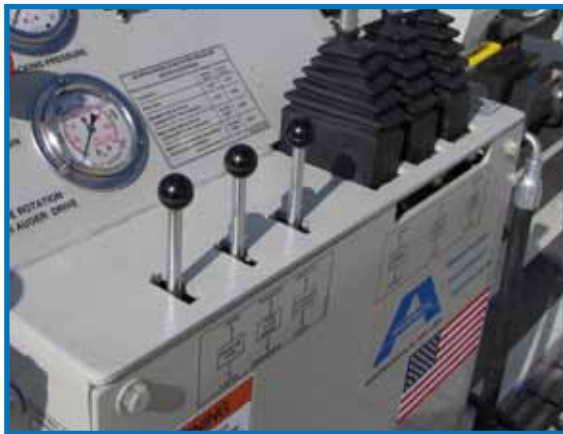
Low pressure valves for hydraulic make-up tool, push plate brake and staging functions.
