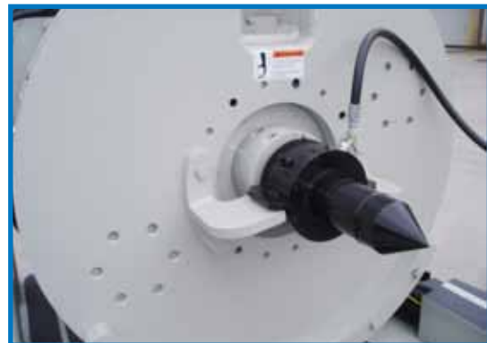
Drive Swivel Adapter With Fluid Connector And Alignment Adapter
