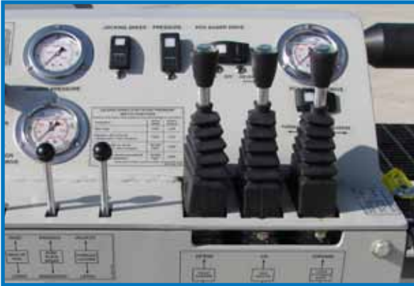
High pressure valves for jacking and rotation functions. Hydraulic pressure gauges for monitoring thrust, rotation and cutter bit system pressures.
