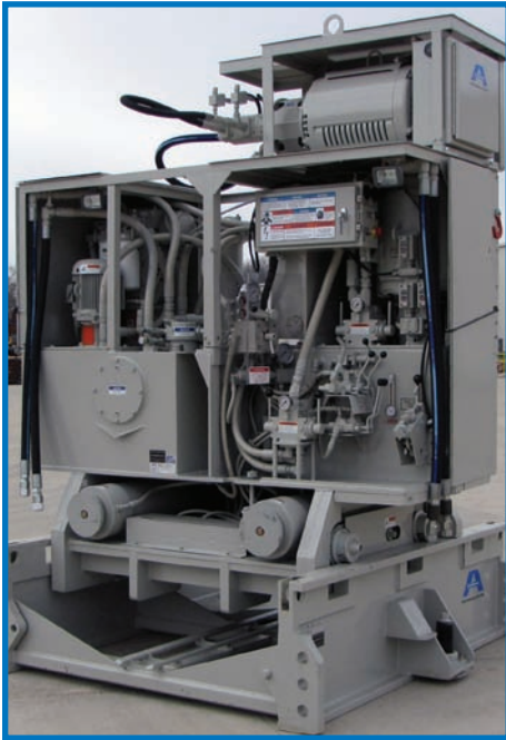
5000 Pump Unit With 100 HP Auxiliary Pump Unit
