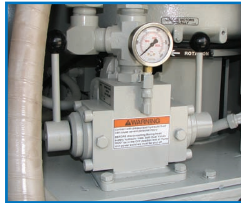
Dual valves control the hydraulic oil flow to the boring head components.
