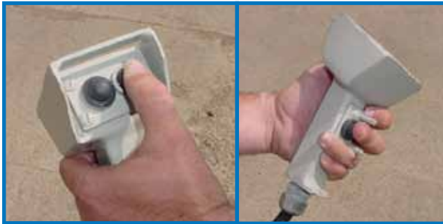
Pendant type controller with propulsion controls and an electric release brake switch.
