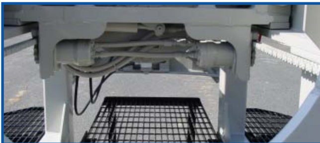
Dual travel motors for ease of advancing gear box along the frame rails.
