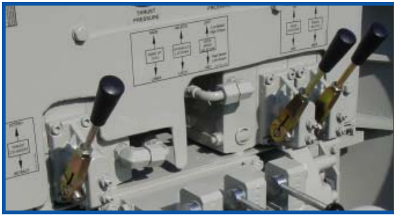
High pressure valves for jacking, rotation, & frame travel functions.
