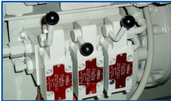
Low pressure valves for hydraulic make-up tool, rotation speed, and hydraulic latching functions.
