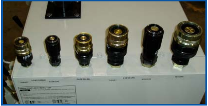
The quick couplers connect to the pressure, return, load sense, and case drain hydraulic hoses from the GBM P100Q Power Pack.
