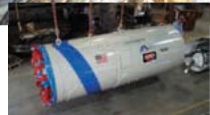
Akkerman SL60 MTBM lowered into one of the nine launch shafts on the Warnimont Avenue relief sewer project
