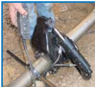
The remote pendant contains the engine tachometer, hourmeter, engine oil pressure gauge, water temperature gauge, electronic engine speed control, and ignition switch.
