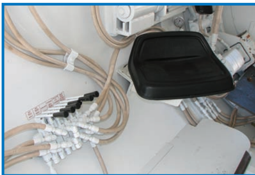
Operator station with six-way control valve. This valve controls the inner drum, conveyor, steering, dirt wing, and closed face doors.
