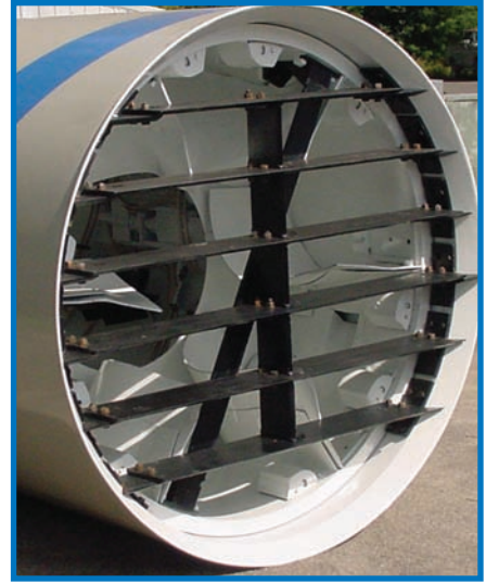
Sand shelf attachment for loose, ununstable soil, but not flowing.
