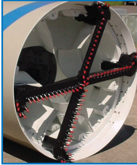
Carbide cutter head attachment for soft to medium hard rock.
