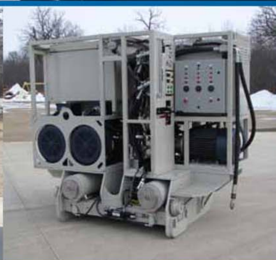
The 5000 Series II Pump Unit features two 100 HP (74kW) low pressure electric motors for TBM and conveyor functions and one 50 HP (37kW) high pressure electric motor for the main hydraulic cylinders and auxiliary jacking functions.
