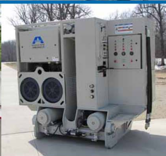
The pump unit is positioned on the back end of the skid, behind the yoke and houses the jacking cylinders and hydraulic power. The operators platform offers a safe location for access to controls.
