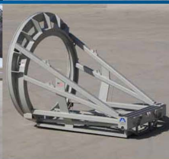
The thrust yoke is pushed by hydraulic cylinders on the pump unit and is sized to match the pipe size. This yoke features extension rings for a larger pipe diameter.
