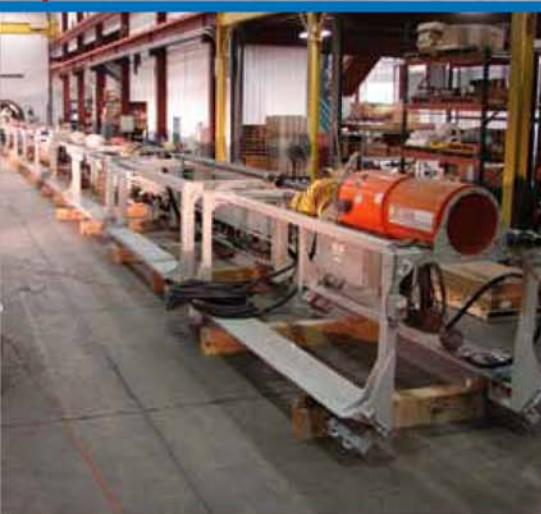
Many specialized back-up cars are needed to perform the complex operations of the segment erecting EPBM.
