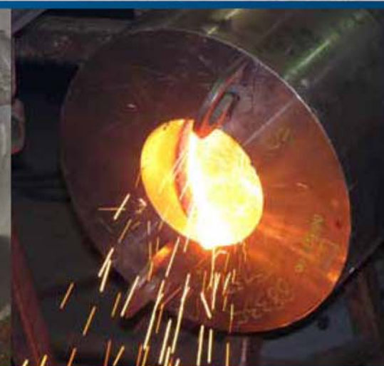
Akkerman custom manufacturers most components for all of our equipment lines. Welding of the EPBM screw conveyor is shown here.
