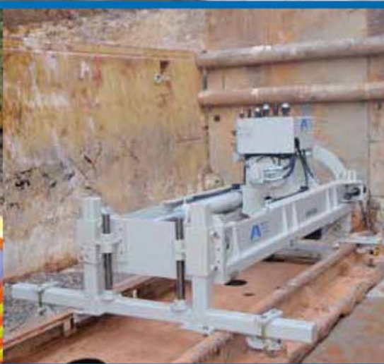
The universal auger bore rig adapter and mounting hardware for the 240A jacking frame fits 30-72 inch (762-1,829 mm) track.
