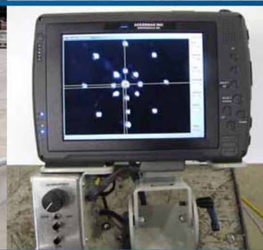
The guidance system provides line and grade accuracy up to 487-feet (150 m) and beyond. The LED target is placed in the first pilot tube and monitored on the tablet computer monitor and mounted to the jacking frame. (Photo cross hairs have been enhanced).
