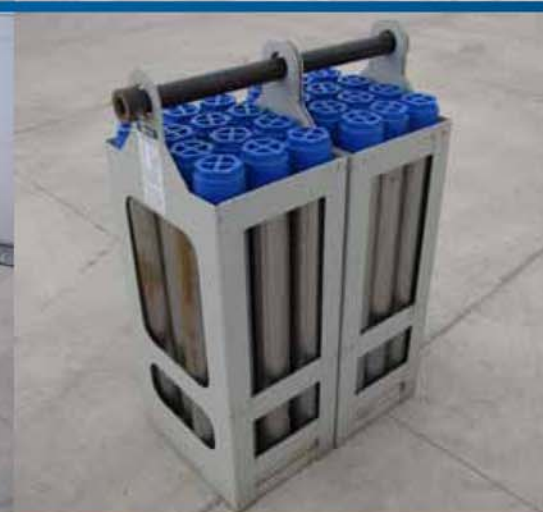
The 30-inch (762 mm) pilot tubes feature a unique dual-walled design. The 2-inch (51 mm) ID inner tube diameter allows for viewing of the target during the drive while the 2.4 square inch annular space (1,548 sq. mm) allows for fluid passage.
