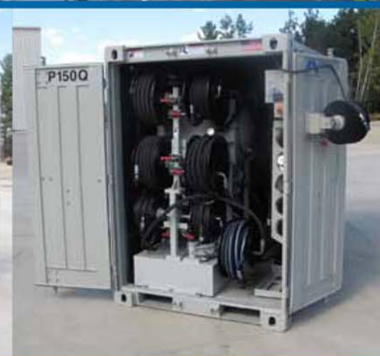
The P150Q Power Pack features a four-cylinder, liquid cooled, 154 HP (115 kW) engine with three variable-piston pumps for independent operation of the jacking, rotation and PCH.
