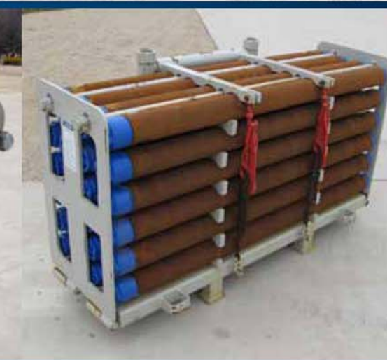
The 60-inch (1,524 mm) pilot tubes feature a unique dual-walled design. The 2-inch (51 mm) ID inner tube diameter allows for target viewing during the drive while the 2.4 square inch annular space (1,548 sq. mm) allows for fluid passage.
