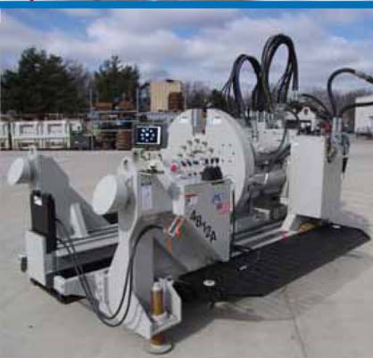
The 4812A frame is capable of installing up to 48-inch (1,219 mm) pipe, two-meters in length. It features independent jacking, rotation and cutter bit operation.
