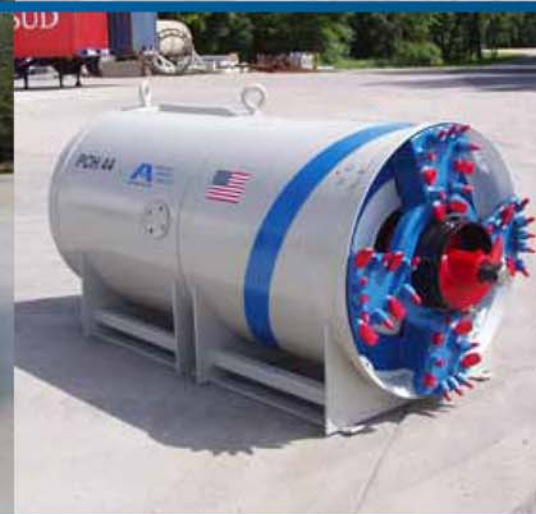
The large diameter PCH 36 and 44-inch OD models (914-1,118 mm) reduce jacking force and lubricate spoils at the face of the bore for ease in removal.
