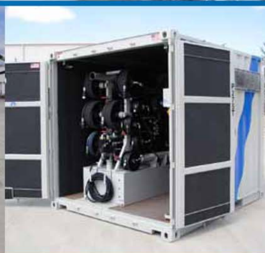
The P275T Power Pack features a six-cylinder, liquid cooled, 275 HP (205 kW) diesel engine with three variable piston pumps for independent operation of the jacking, rotation and PCH.
