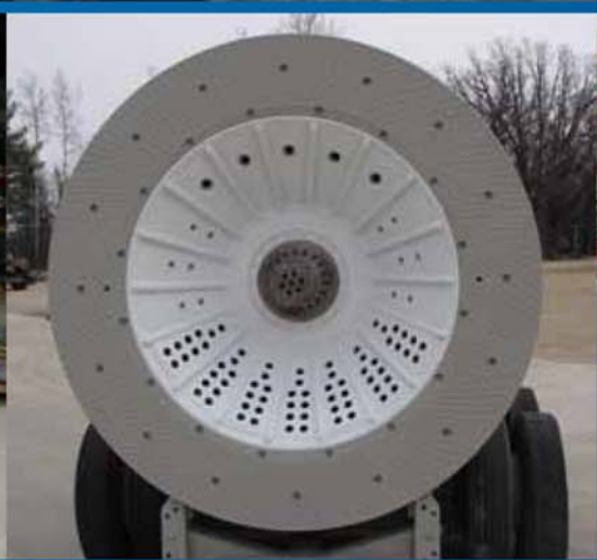
With the cutter face removed, the crushing cone's slurry inlet holes, high pressure jetting nozzles and spoil intake ports are clearly visible. This MTBM SL74 has been skinned to 102-inches (2,591 mm).
