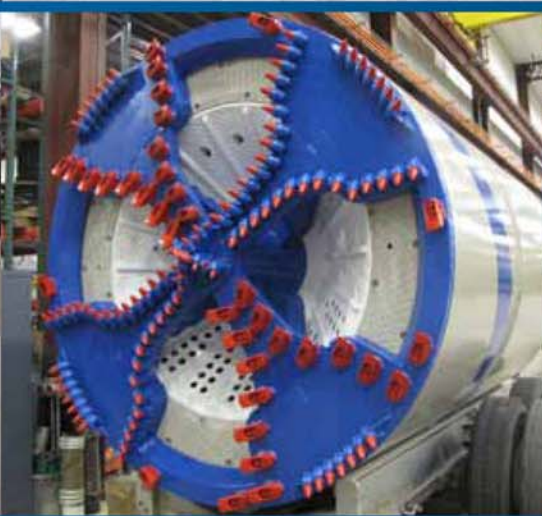
Our MTBMs can be equipped with the appropriate cutter face for job requirements. Shown here is the soft ground configuration featuring a combination of carbide drag and bullet bits.
