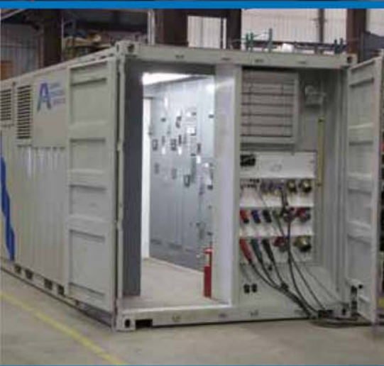
The Control Container is the information center for all microtunneling functions. It houses the control console, motor control centers for slurry pumps, MTBM drive motor and the bulkhead panel for electrical and communications connections.
