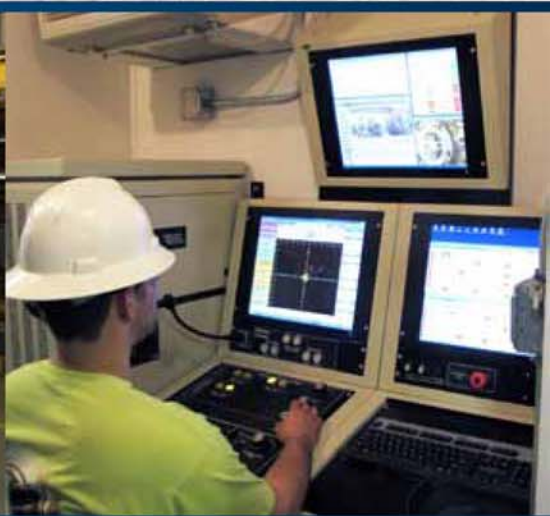
The MTBM operator maintains control of all microtunneling functions during operation from a three-monitor console in a climate controlled environment.
