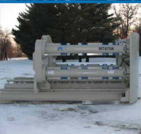
The MT875K operates out of a mere 20-foot (6.1 m) shaft while jacking pipe with 800 tons @ 8,000 psi (726 mt @ 550 bar) of force.
