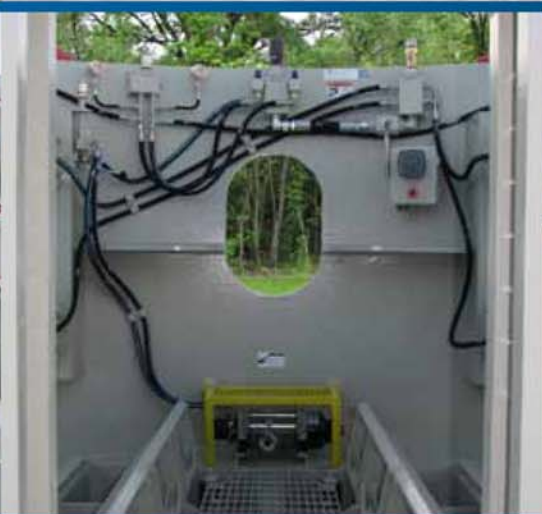
The laser guidance slot is visible here along with the frame's hydraulics and the winch pullback for the thrust block.
