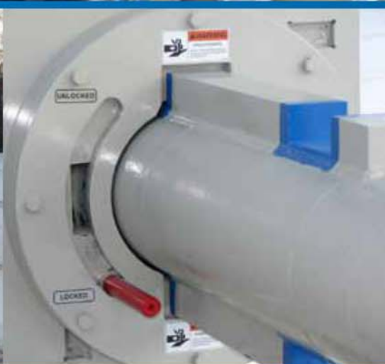
The keyhole jacking frames feature keyed blocks on the jacking cylinders to continuously advance the machine.
