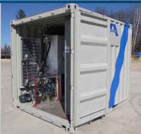
The Remote Hydraulic Power Pack houses a 27 gpm @ 8,000 psi (550 bar) high pressure pump. The main displacement pump contains a 150 HP (112 kW) electric motor and variable frequency drive for output flow control.
