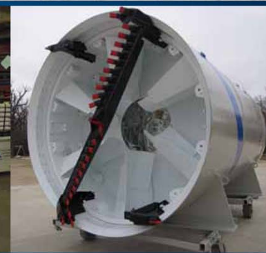
Akkerman TBMs are equipped with three cutter head configurations. Cutter heads can be changed underground as soil conditions vary. The dirt cutter head is pictured here.
