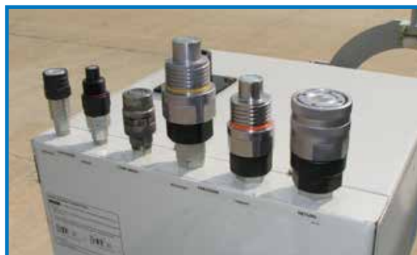
The quick couplers connect to the pressure, return, load sense, and case drain hydraulic hoses from the GBM Power Pack.
