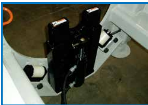
The hydraulic make-up tool is used to tighten each section of the pilot tubes as they are installed in the launch shaft. In pull back operation, the make-up tool is used to separate the pilot tubes in the launch shaft.
