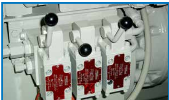
Low pressure valves for hydraulic make-up tool, rotation speed, and auxiliary functions.
