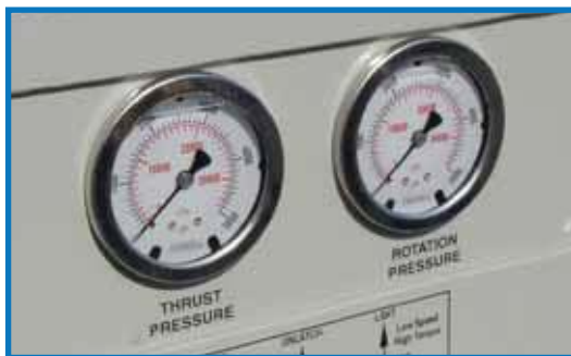
Hydraulic pressure gauges for monitoring thrust and rotation system pressures.
