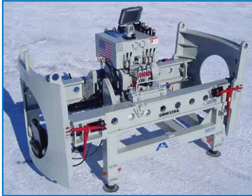
The GBM 339A latching frame is shown with round shaft adapters.
