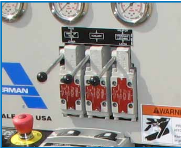
Low pressure valves for hydraulic make-up tool, auxiliary and latching functions.
