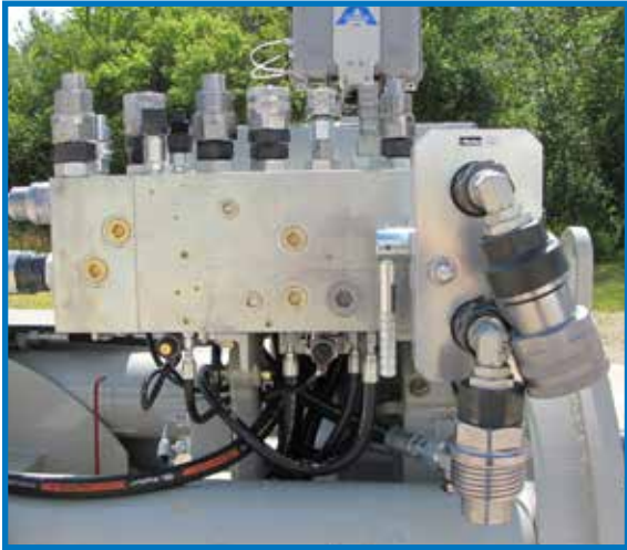
The quick couplers connect to the pressure, return, load sense, and case drain hydraulic hoses from the GBM Power Pack, along with the PCH hydraulic hoses.
