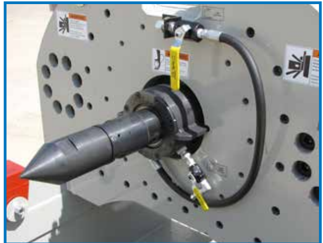
Drive Swivel Adapter With Fluid Connector And Alignment Adapter
