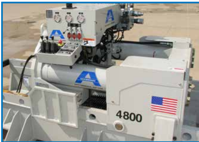
Two 40 inch stroke cylinders provide up to 265 ton thrust capacity.
