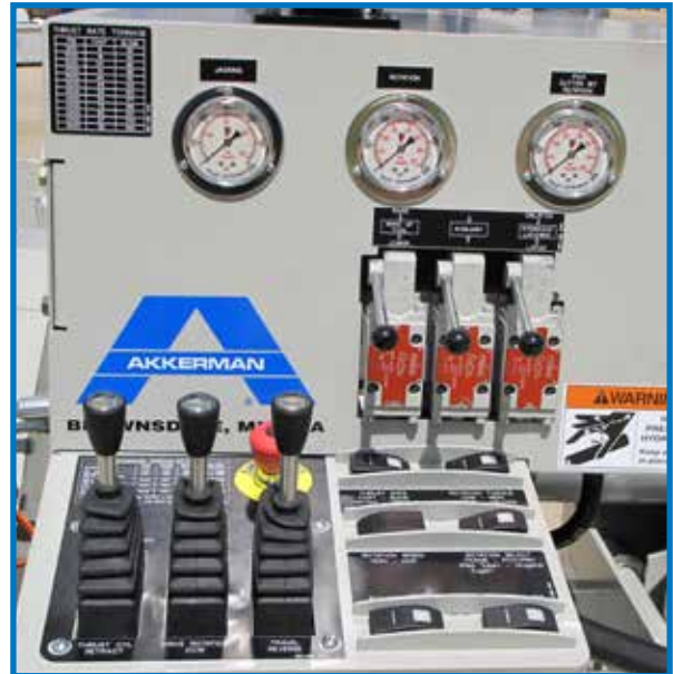
High pressure valves for jacking and rotation functions. Hydraulic pressure gauges for monitoring thrust, rotation and cutter bit system pressures.
