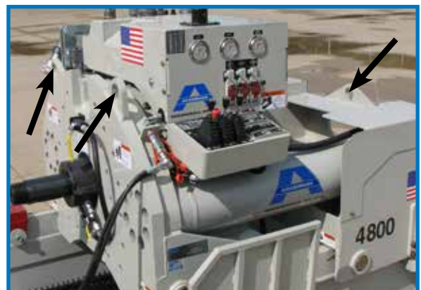
Three thrust frame lift points for ease of repositioning thrust frame.
