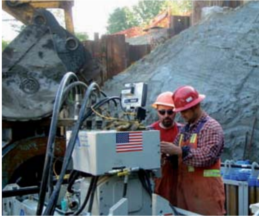
Kamloops owns two Akkerman guided boring machine (GBM) pilot tube systems
