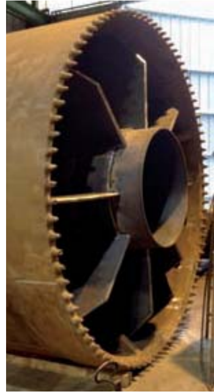
Kamloops used a 3,048mm weld-on reaming head to upsize to the 3m OD steel pipe culverts
