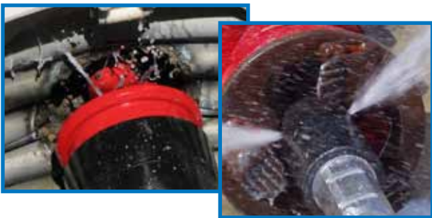
For efficient and productive operation of the swivel cutter head, there must be a minimum jetting supply of 16 gal @2,500 psi.
