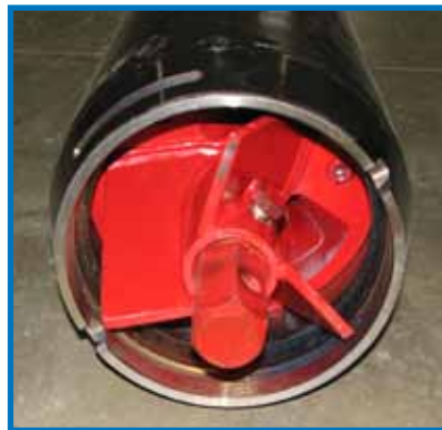
Cutter head with drag and conical bullet bits.
