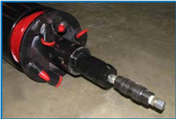
A fluid connector is equipped on the swivel cutter head permitting lubrication of the spoils to reduce jacking forces.
