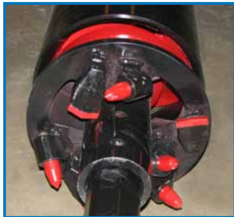
Cutter head with drag and conical bullet bits.
