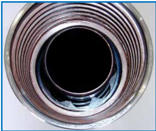
Each pilot tube contains a valve assembly that restricts the fluid from flowing during the installation of the next pilot tube. Fluid can be supplied from the launch shaft or the reception shaft depending on the job requirements.
