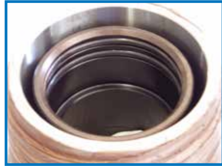
Dual o-rings at the inner tube seals the connection between the pilot tubes. The inner tube is treated to resist corrosion assuring a good seal at the mating surface to the o-rings.
