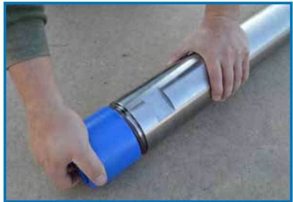
Pilot Tube Cap And Plug Maintains clean lubrication of the thread joint between pilot tube use. Protects the o-ring sealing on the inner tube while in storage. The thread joint can be lubricated as the pilot tubes are removed so they are ready for the next drive.
