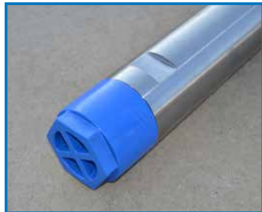
To lock and unlock the pilot tubes, two parallel dual slots are located on each end of the pilot tube to work in conjunction with tooling on the jacking frame.
