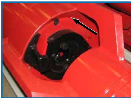
Jetting Ports (2) On Reaming Head Arms
