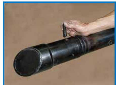
Double Pinned For Ease Of Changing Steering Heads
