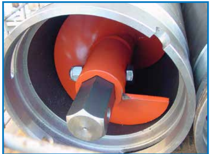
2 or 3 Inch Hex Connector Bolted To Auger
