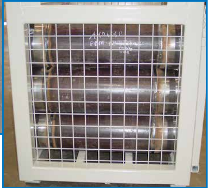
Wire Basket Carries Augers & Casings.
