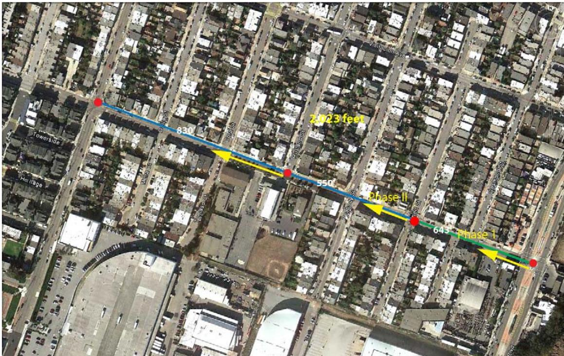
Figure 1: Microtunneling drives and shaft locations.
