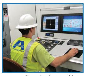
Operator can easily monitor the status of the target, control, indicator screen displays and control all system components from inside the Control Container.
