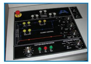
The slurry removal system, steering, cutting head, jacking frame, and emergency stop controls are located on the control console.
