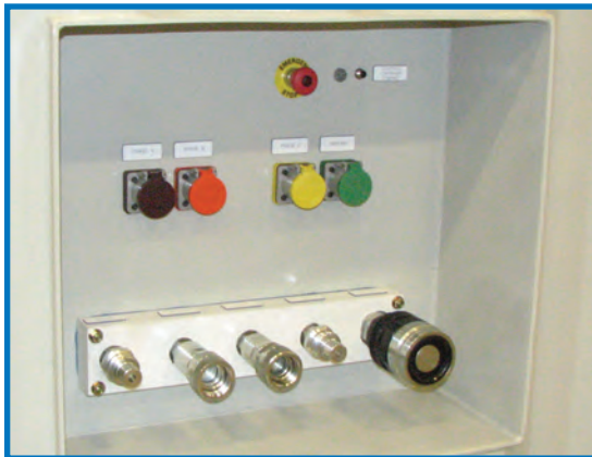
Bulkhead Panel For Electric, Hydraulic, Communication Connections & E-Stop Button
