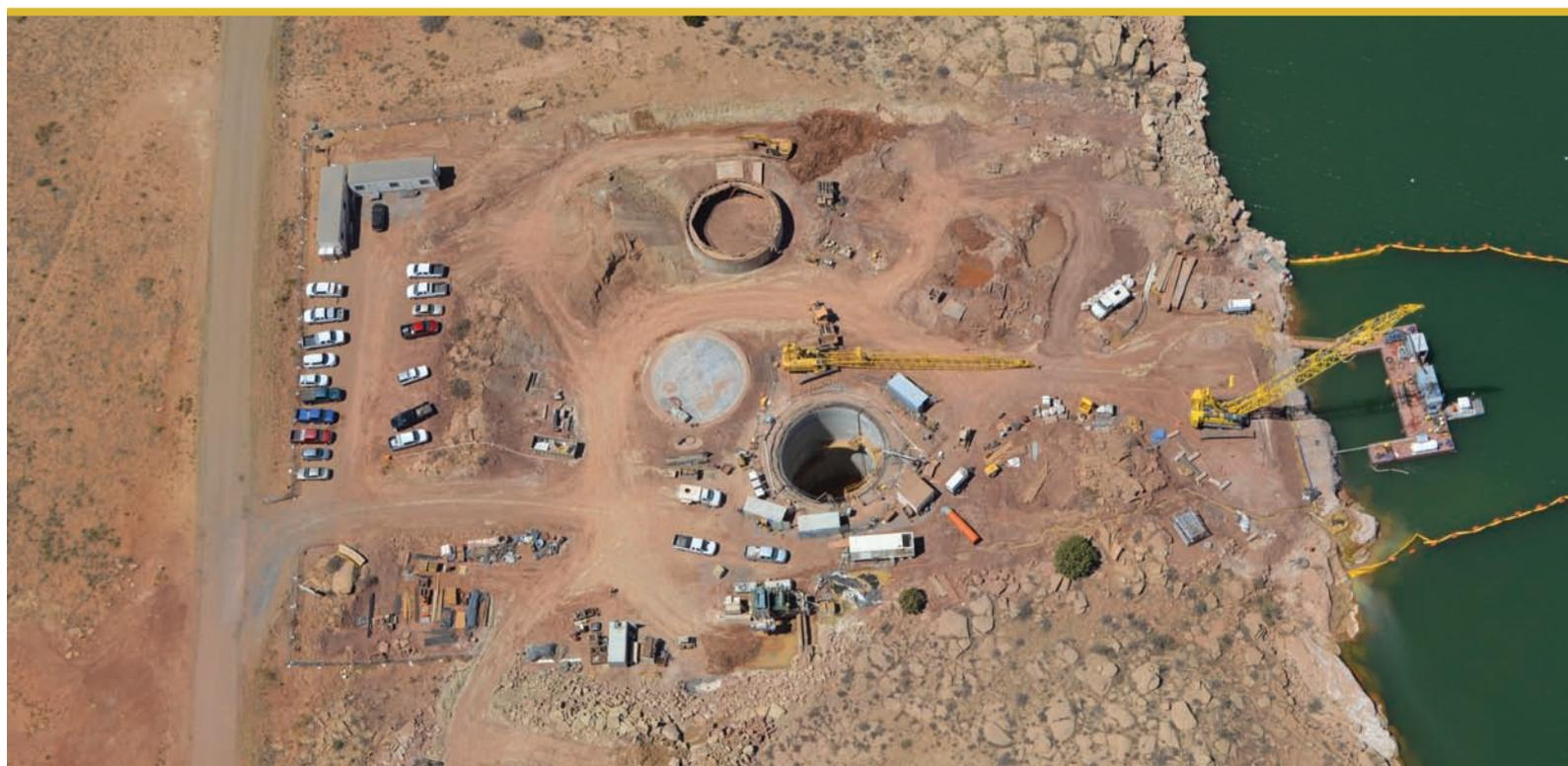
**NADA PACIFIC RECENTLY COMPLETED A 60-IN. DIAMETER, 236-LF MICROTUNNEL INTO UTE RESERVOIR IN NEW MEXICO.**
