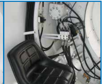
Operator station with pilot operated controls for the inner drum, conveyor, and auxiliary functions.
