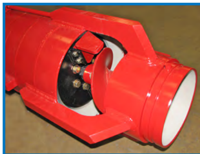
Auger Chamber Shears Spoils Away From Cutting Ring To Reduce Jacking Forces
