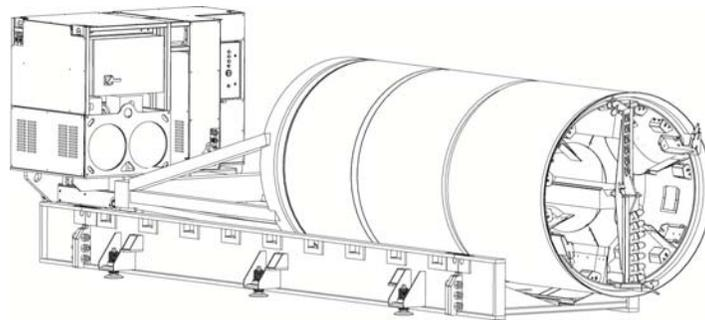
Figure 7. All-in-one pipe jacking system.
