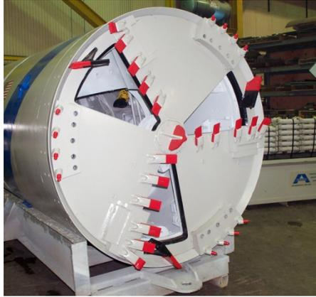
Figure 4. A closed face cutter head prevents spoils from entering the interior of the TBM and has the option to close the entire face.
