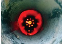
One of the most common applications for the single stage **GBM 240A Jacking Frame System** is its use in conjunction with a standard auger boring machine to install steel casing pipe. With the GBM providing guidance, contractors are empowered with the possibility for longer drives, extreme accuracy and reduced casing diameters. In addition, using a GBM 240A system can also serve as a probing tool for uncharted obstacles with minimal commitment to the bore.
