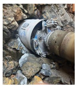
however the transition can be affixed to a myriad of head types including Rock Boring Units (RBU's). When using a retractable type of ABM cutterhead during this stage, the upsize bearing assembly will allow the operator to trip augers and repilot the bearing assembly for continued operations.
