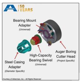
The robust 100-ton upsize bearing package includes a Steel Casing Adapter that pilots inside the first casing upsize (16-30 inch). The bearing assembly affixes to an ABM cutterhead of the contractor's choice by attaching it to the Bearing Mount Adapter ring located at the center of the face plate. A retractable type Akkerman cutterhead is shown in the illustration,
