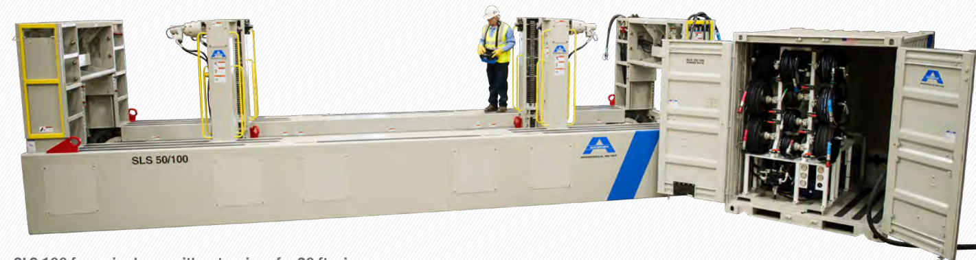
SLS 100 frame is shown with extensions for 20-ft. pipe
