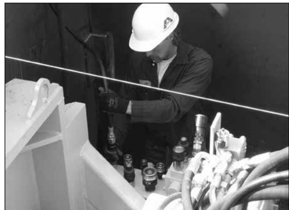
GBM Hydraulic Connections
