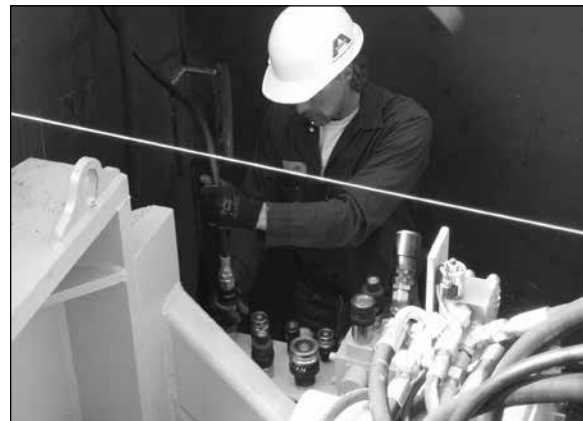
GBM Hydraulic Connections
