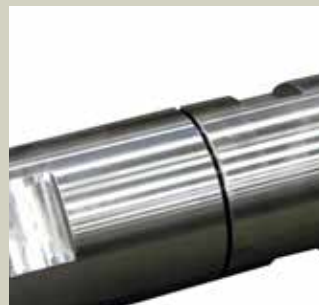
Figure 3. Good, smooth pilot tube connection.
