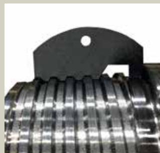
Figure 1. Pilot tube presenting a good thread wear pattern.
