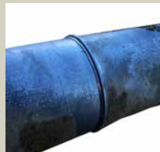
Figure 4. Pilot tube connection presenting ballooning.
