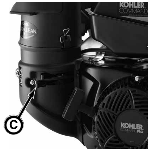
Engine Fuel Shutoff Shown in Off Position
