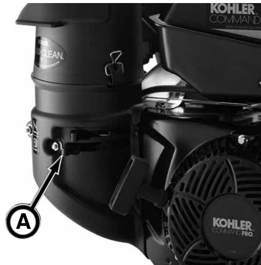
Engine Fuel Shutoff Shown in Off Position
