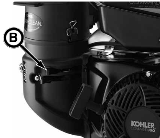
Engine Choke Control Shown in On Position
