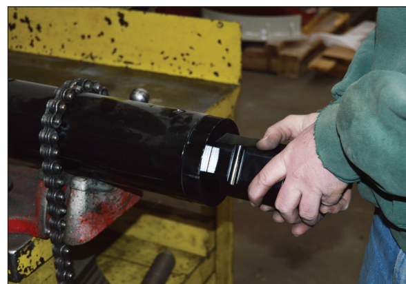
Inspecting Bearing Swivel Assembly For End Play
