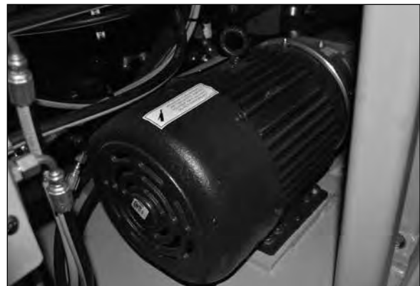
5 HP Electric Motor
