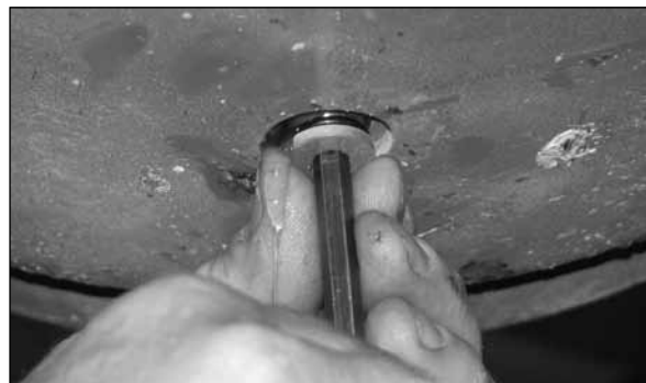
Loosening Drain Plug For Sample
