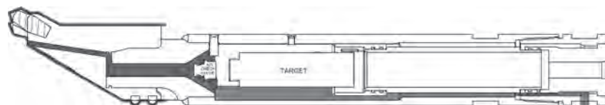
Pilot Tube To TriHawk Adapter (RDA) With TriHawk Drill Bit Fluid Path
