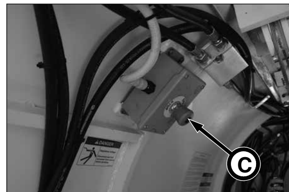
E-Stop on TBM
