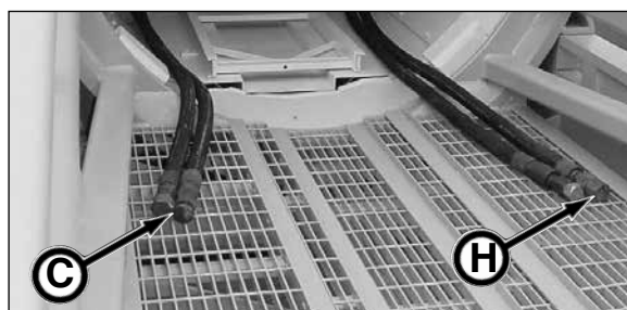
TBM Supply & Return Hoses
