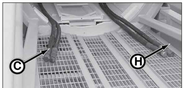
TBM Supply & Return Hoses
