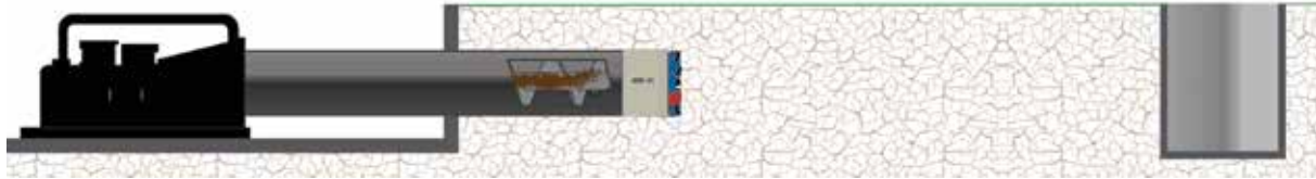
RBU Installation With Auger Boring Machine
