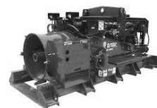
Auger Boring Machine
