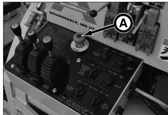
4800C Control Console Emergency Stop Button
