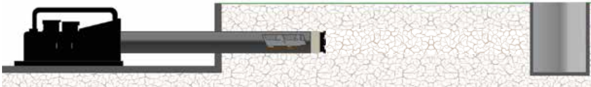
GRS-50 UnGuided Installation With Auger Boring Machine
