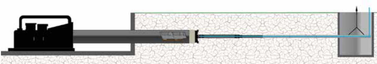
GRS-50 Guided Installation With Auger Boring Machine
