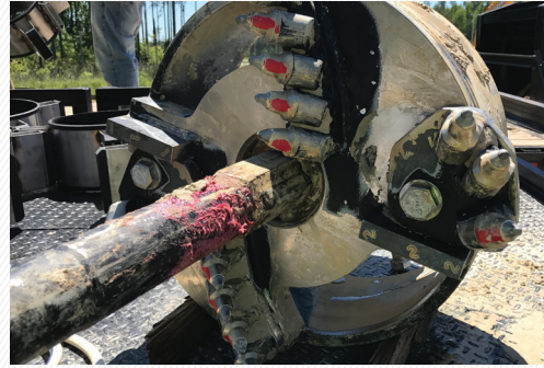
Figure 10. Swivel, guide rod and cutter head all-in-one.
