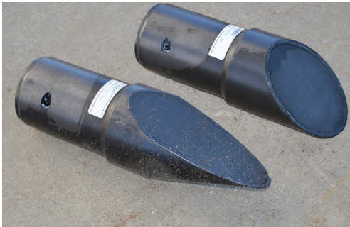
Figure 2. A bullet steering head is used for high blows count ground and a blunt, 45-degree steering head is used for soft ground conditions.
