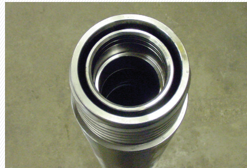
Figure 1. Dual-Wall Pilot Tubes allow for fluid passage to the steering head through an outside ring and visibility of the guidance system's target in the inner tube chamber.
