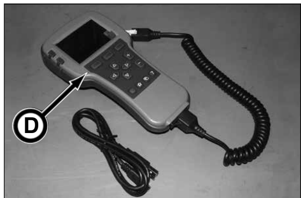
A handheld diagnostic tool P0304-324A with a blue band is compatible with the Drive Motor Controller SN F21700F 29 & after.
