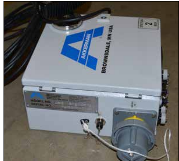
ABIS Remote Station Control Box
