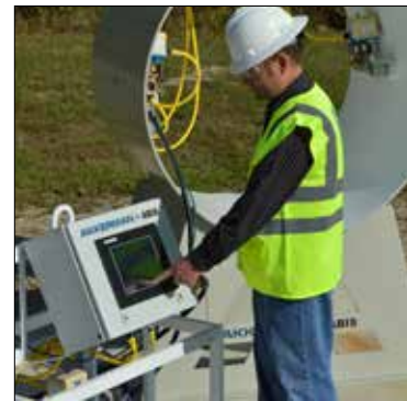
Akkerman Bentonite Injection System (with Simulated Tunnel Pipe)
